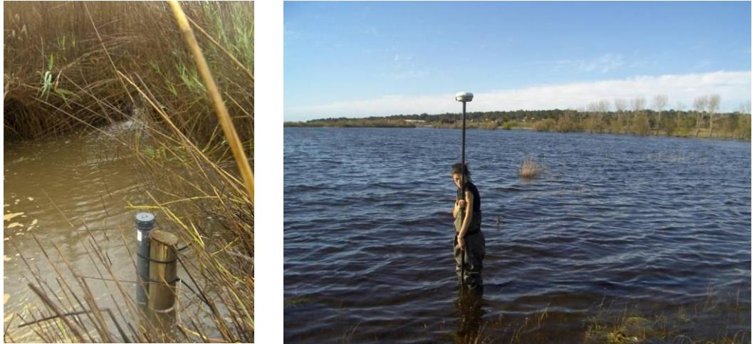
**Figure 15.** Installed CTD in the SAL (left) and lagoon water level measurements using a DGPS.
