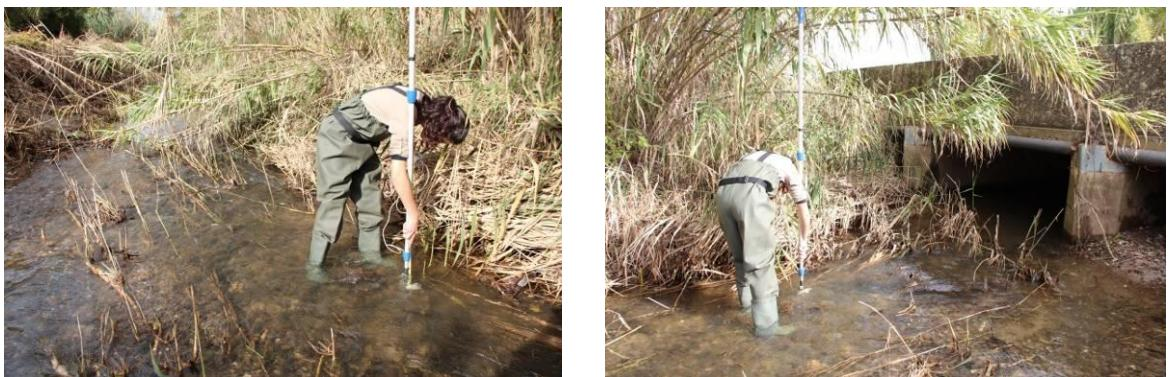
**Figure 3.** Velocity measurements photos at SR3 location, before stream bed changes.
