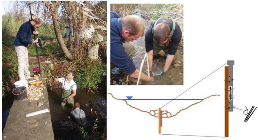
**Figure 2.** Streams CTD installation schema (right down corner) and SR1 (left) and SR3 (right) CTD installation photos.
